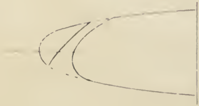
LEADING EDGE NO. 5 SAME AS CONTOUR NO. 1 SLOT ADDED REF. DWG. W.T. 179-96 5 OF 7
